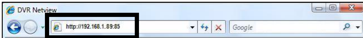
Figure 15.4 Enter :85 at the end of the IP address
